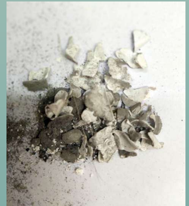
EVA encapsulant separated from the panel using thermal methods (heated up to 60%)
