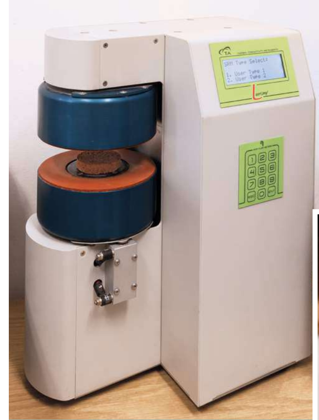
A stationary heat flow meter to study the efficiency of the heat transfer coefficient of materials made of clay and used coffee within the range between 0,1 W/(m·K) and 10 W/(m·K)
