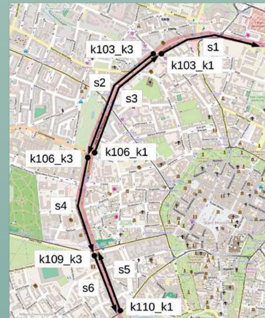
The scope of the dynamic lighting control system (the map shows the northwest bypass of the Krakow city centre) and a fragment of the control graph that manages the data from sensors with dimming parameters of lamps
